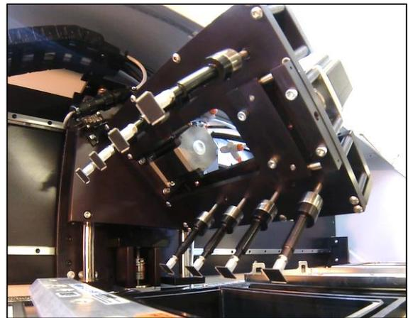
*RPS Lead Tinning Rotary Head running an 8-up QFP process on the Odyssey Lead Tinning System.*
