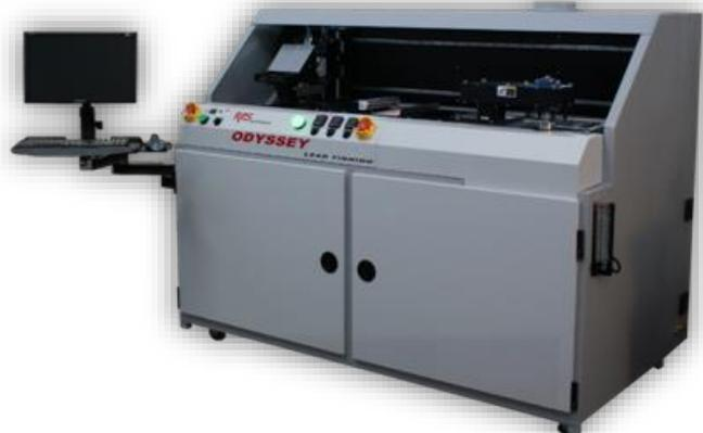
The new alloy station features a high-capacity 5 x 8" (125 x 200mm) nitrogen inerted solder bath that recirculates the solder for a dynamic laminar flow and superior solder application to component terminations. Compared to hand dip tinning or decades old systems that utilize static non-flowing solder baths, the performance of an RPS system represents a many-fold leap in quality and consistency of the tinning process.
